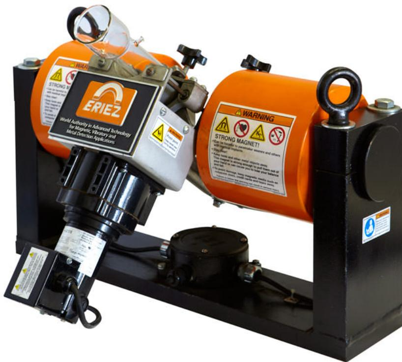
**Figure 1. Typical Davis Tube Recovery (DTR) Measuring Device**
